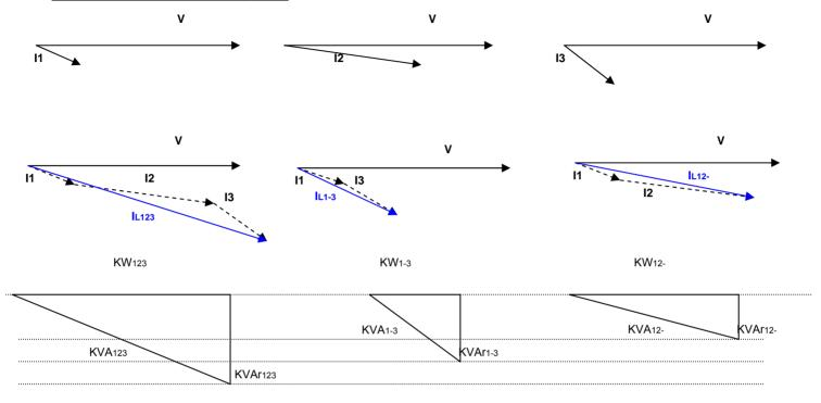
The situation above shows that variable kVAr compensation is needed for various loading conditions.
