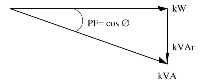
Power Factor is Real (Actual) Power divided by the Apparent Power. i.e. kW/kVA = PF.
